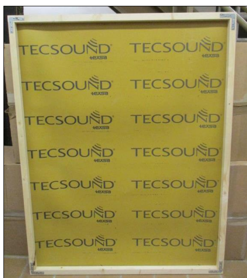
Images 4 to 6 Test element assembly: membrane with wooden frame and perimeter sealing
