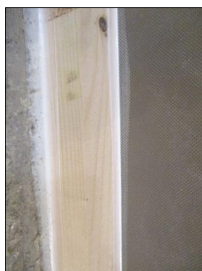
Images 4 to 6 Test element assembly: membrane with wooden frame and perimeter sealing
