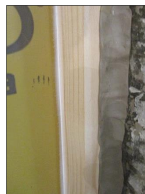
Images 4 to 6 Test element assembly: membrane with wooden frame and perimeter sealing
